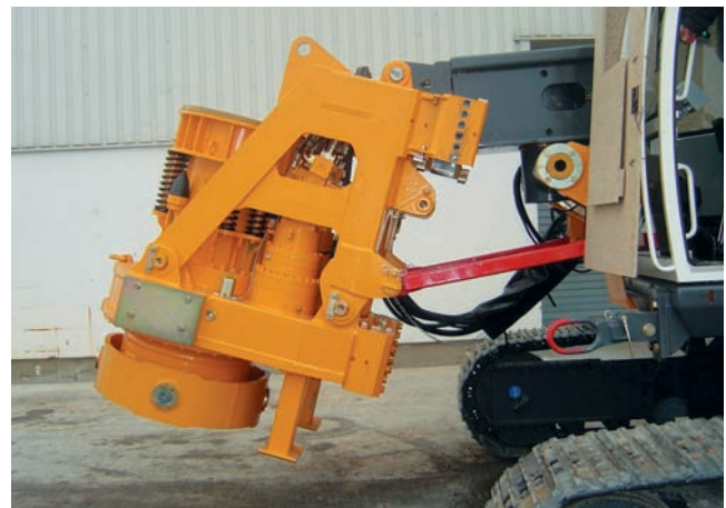
Drehgetriebe in Transportposition (hydraulische Bolzenverbindung zum Mast und Transportsicherungsstangen (rot)) rotary drive in transport position (connected with hydraulically actuated pin to mast and secured with steel beams (red))
