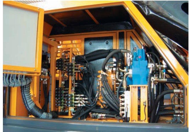
servicefreundliche Hydraulikinstallation service-friendly hydraulic installation
